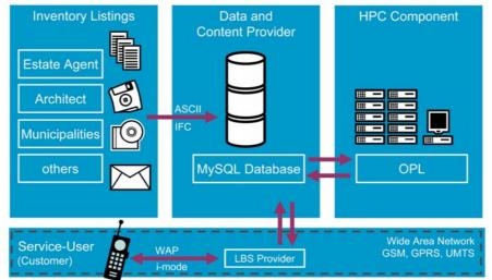
Figure 4. Data transfer and communication.
